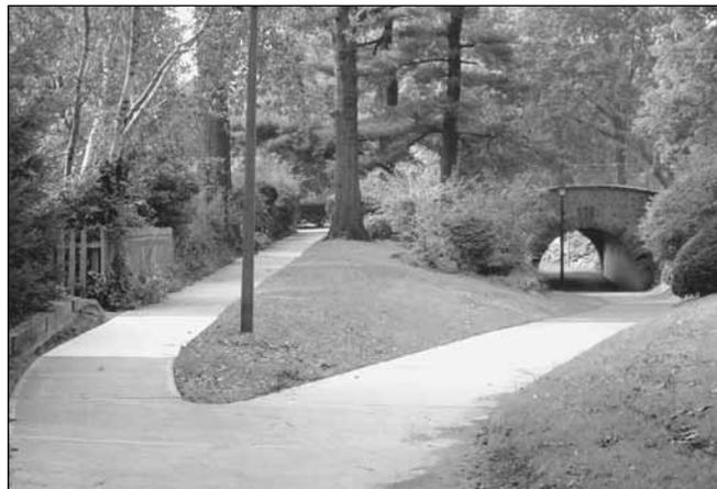
Pedestrian traffic is separated from automobile traffic in Radburn through a carefully designed system of overpasses and underpasses.
