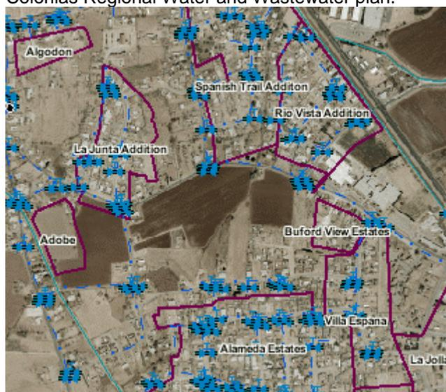
Figure 3. Water and wastewater lines in El Paso, Texas.
