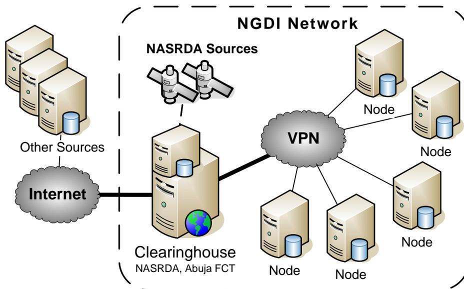
Figure 4: The NGDI Network Supports Distributed Holdings with a Common Clearinghouse.
