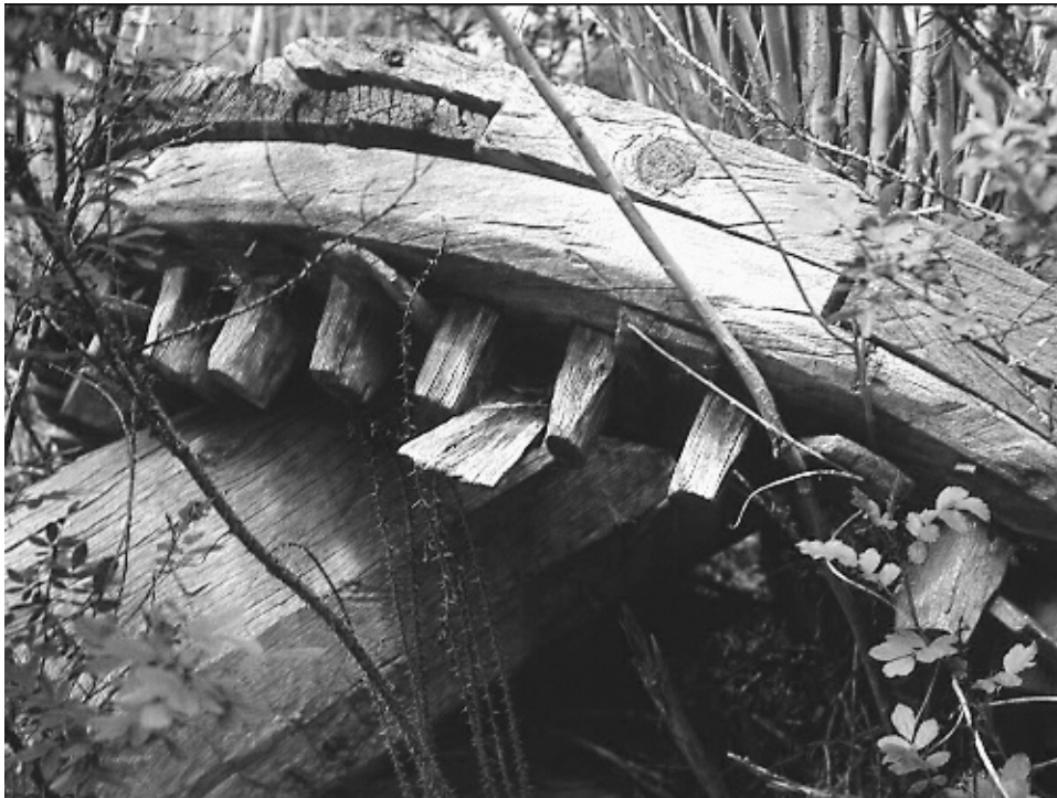
Figure 1: This wheel from an arrastra, built in the Spanish-Mexican technique, was turned with water diverted from a creek along the California-Nevada border, and likely hasn't been seen by more than a couple of dozen hearty bikers in the last fifty years. Made from mountain mahogany and bristlecone pine, it survives and raises questions: Who built it, and why don't we know their history?
